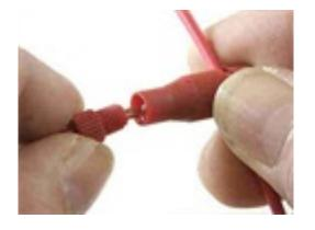
Insert the wire strands into one side of the metal core.
