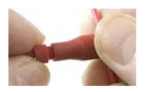
Push and turn until the threads catch, then screw in tightly by hand - make sure the wire does not slip back in the cap
