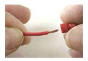
Unscrew the cap and insert the wire end. Be careful to get all the strands through the cap.
