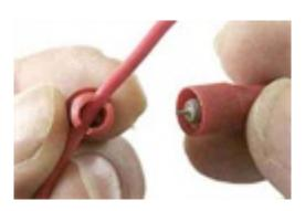
Slide the large cap over the wire as far as it will go. Here, the wire to be tapped is inserted and ready to tap.
