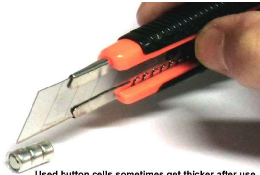
Used button cells sometimes get thicker after use. Slit the insulation and then put in 3 new batteries.
